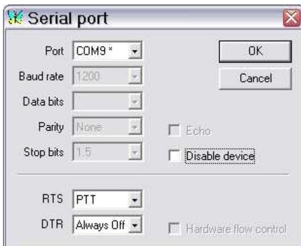
5. Click **Configure | FSK Port | Port Settings** (if your radio does not support FSK, click Configure | Secondary PTT Port instead).
